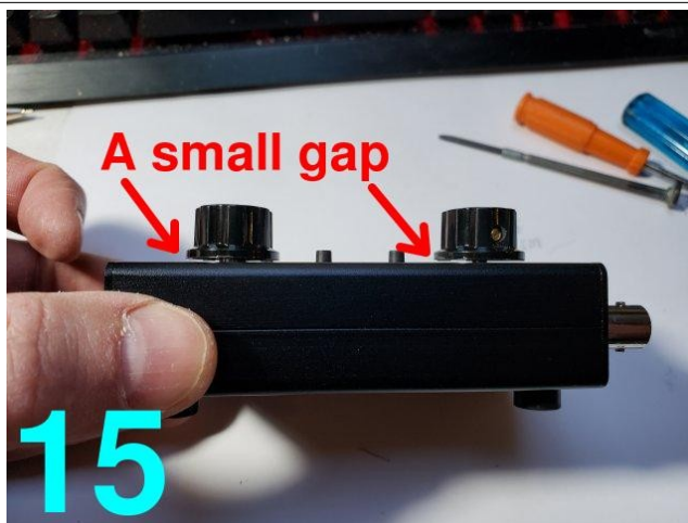
15 Install the supplied knobs by tightening their grub screws. Leave a small gap between each knob and the front panel, to allow the knob to turn easily. The grub screw of the volume control knob should be at the position of the flat on the shaft. The grub screw position on the rotary encoder is not important.
