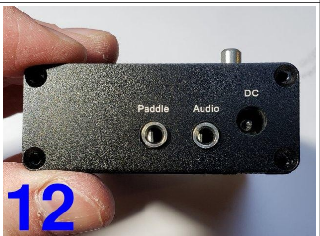
12 Now bolt the left-hand side panel to the enclosure extruded top and bottom halves using four of the supplied small black countersunk screws in the panel corners. The screws need to be carefully aligned and should screw in easily (if properly aligned).
