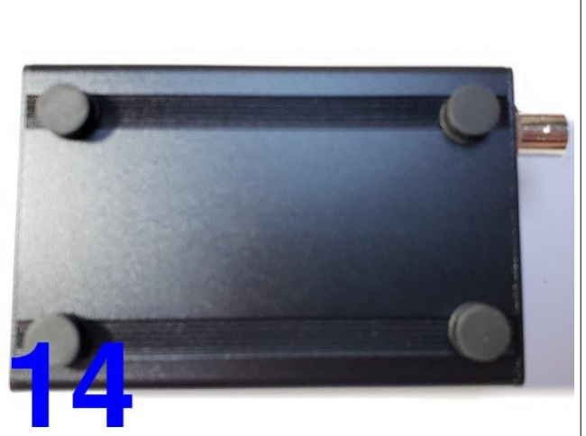
14 Apply the supplied four self-adhesive feet to suitable positions on the base of the enclosure if desired (optional).
